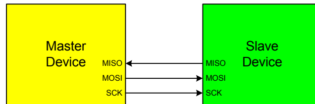
Figure 17.3. 3-Wire Single Master and 3-Wire Single Slave Mode Connection Diagram
